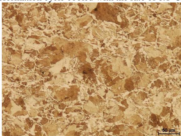
Fig. 5. Ferritic-pearlitic microstructure of the specimen made of 30MnB4 steel after a deformation cycle cooled with the rate of 5°C/s
