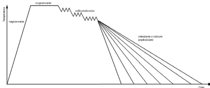
Fig. 2. The scheme of thermal-plastic processing carried out in this work using deformation dilatometer DIL 805A/D
