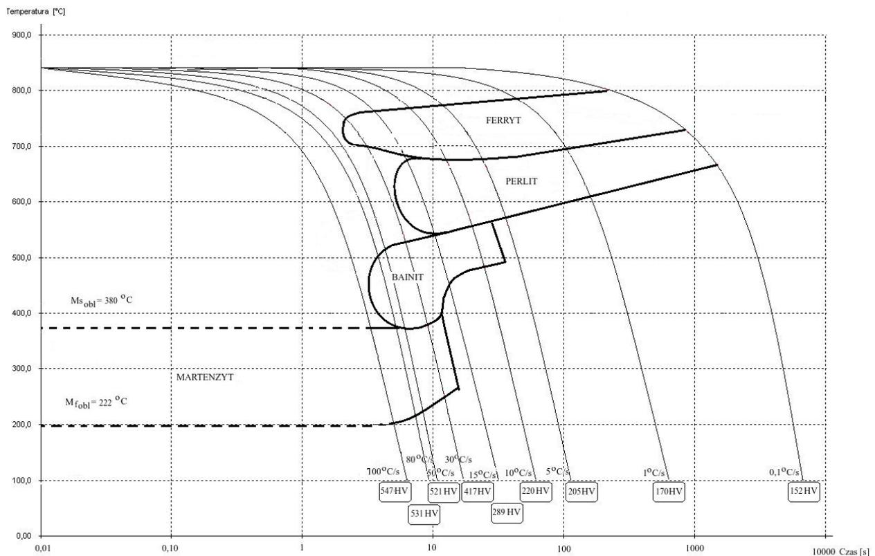
Fig. 11. The DTTT diagram for 30MnB4 steel worked out on the basis of dilatometric tests
