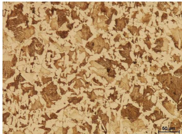
Fig. 4. Ferritic-pearlitic microstructure of the specimen made of 30MnB4 steel after a deformation cycle cooled with the rate of 1°C/s
