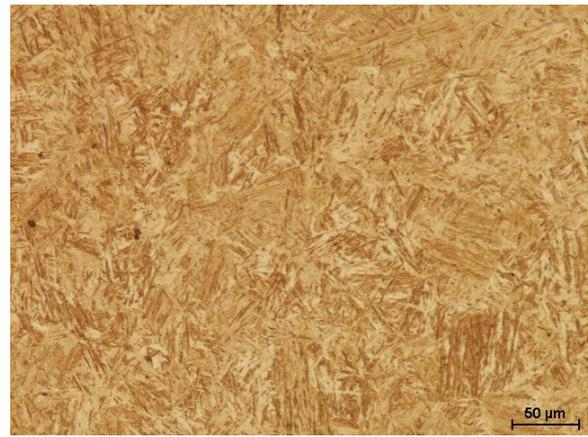
Fig. 8. Martensitic structure of the specimen made of 30MnB4 steel after a deformation cycle cooled with the rate of 100°C/s
