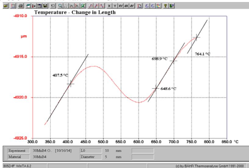
Fig. 10. A dilatograph registered for 30MnB4 steel cooled after deformation from the temperature of  $T_D=830^\circ\text{C}$  with the rate of 15°C/s
