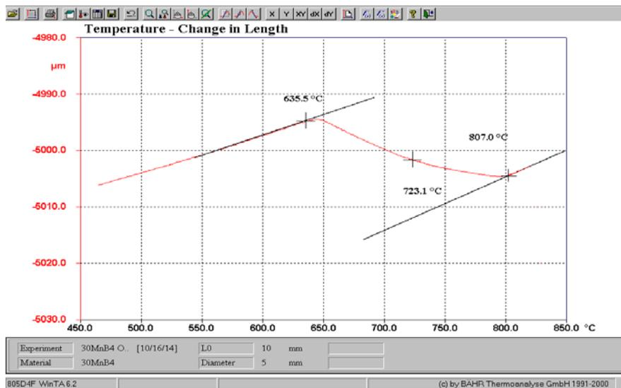
Fig. 9. A dilatograph registered for 30MnB4 steel cooled after deformation from the temperature of  $T_D=830^\circ\text{C}$  with the rate of 1°C/s
