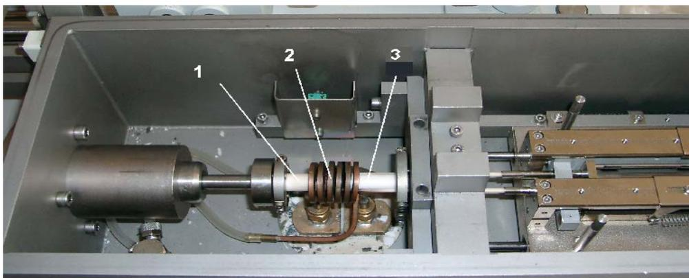
Fig. 1. The chamber of deformation dilatometer DIL 805A/D (1 – movable ceramic anvil; 2 – induction coil, 3 – ceramic anvil)
