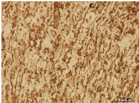
Fig. 3. Ferritic-pearlitic microstructure of the specimen made of 30MnB4 steel after a deformation cycle cooled with the rate of 0.1°C/s
